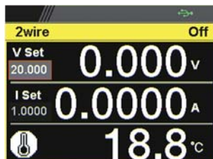
White: Temperature Control on with GTL-205A Connected
